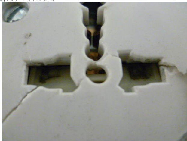
Sample 2 after 10,000 insertions
