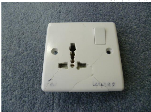
Sample 2 after 10,000 insertions
