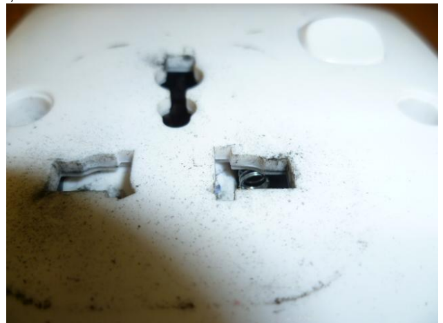
Sample 1 after 10,000 insertions
