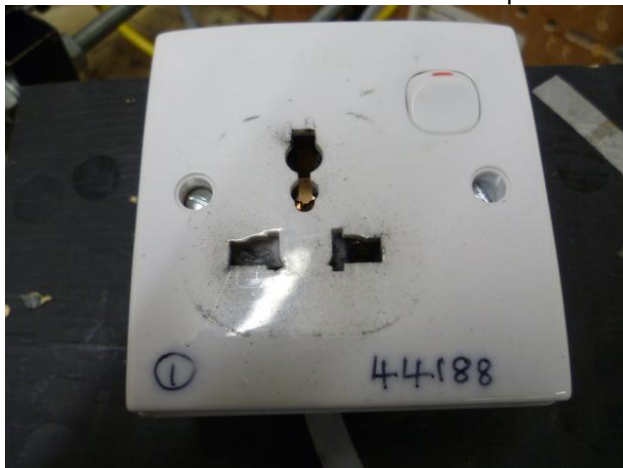
Sample 1 after 10,000 insertions
