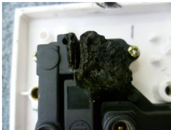
Sample 4 Front plate @ 850°C
