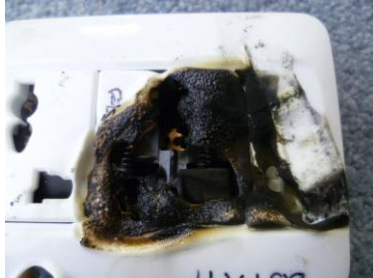
Sample 4 Front plate @ 850°C
