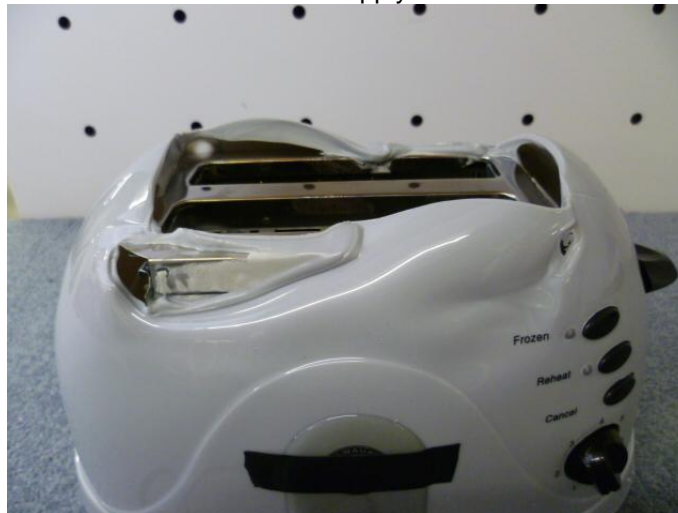
Photograph of 110v toaster after connection to 240v supply
